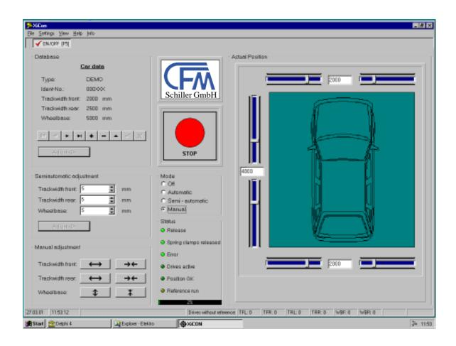
The X-Y-positioners for full car test rigs and 4-poster test rigs are equipped with a PC control system. Our software XiCon allows the automatic as well as semiautomatic and manual adjustment of the positioner units according to various vehicle dimensions.
