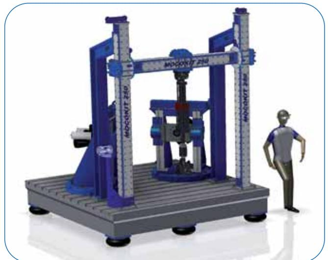
A multi axial test configuration with **MOCOKIT® 250**
