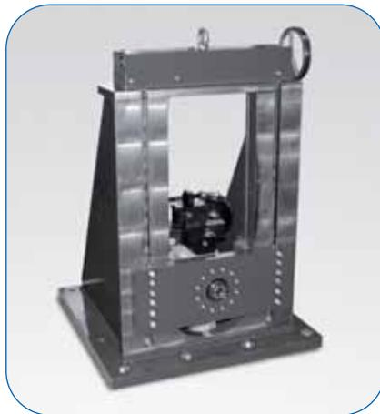
Actuator flange plate for fixed support
