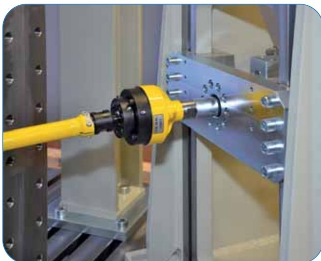
Fixation of height adjustable clamping bracket by means of a bolted connection
